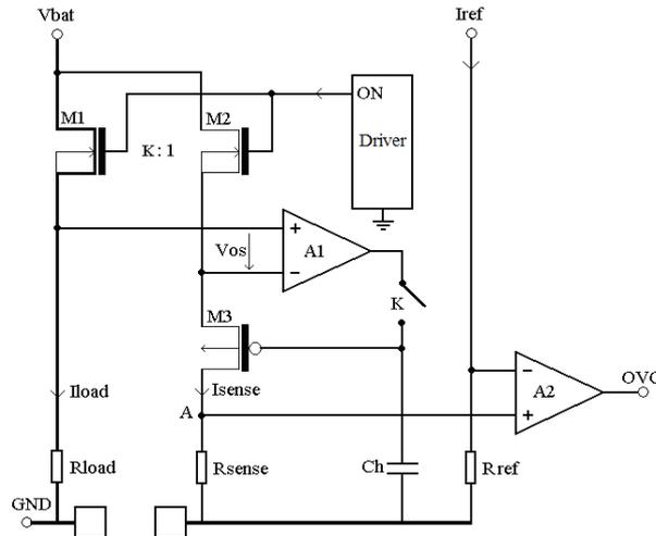
Fig. 3. Over current detection.
