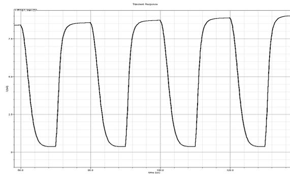
**Fig. 6.** Sense current without the S/H circuit.
