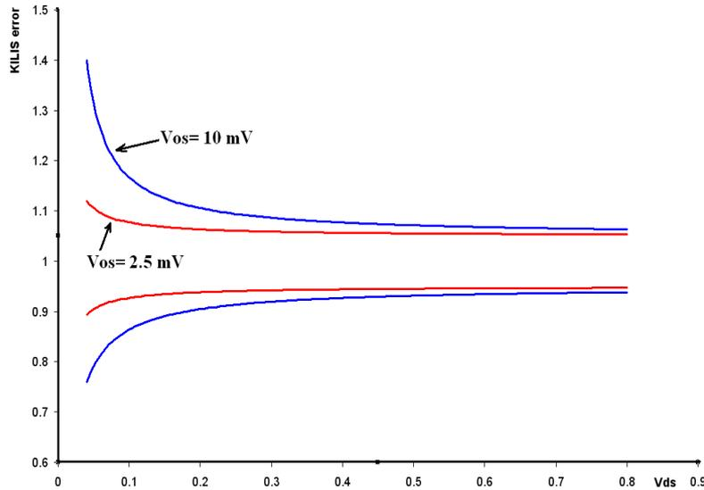
Fig. 4.  $K_{ILIS}$  accuracy dependence on output transistor drain – source voltage.
