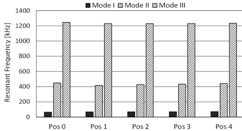
Fig. 9. Resonant frequency as a function of the electrode position for different oscillation modes in air.
