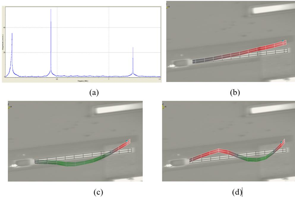
**Fig. 5.** Dynamic response of the polysilicon microcantilever (position - 0) under different bending modes tested in vacuum ( $7 \times 10^{-4}$  mbar): (a) the frequency response curve; (b) the 1<sup>st</sup> mode; (c) the 2<sup>nd</sup> mode; (d) the 3<sup>rd</sup> mode (color online).
