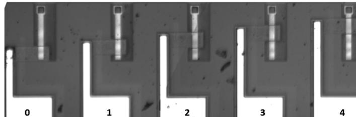
Fig. 4. Resonator microcantilevers with electrostatic actuation and different position of the acting electrode.
