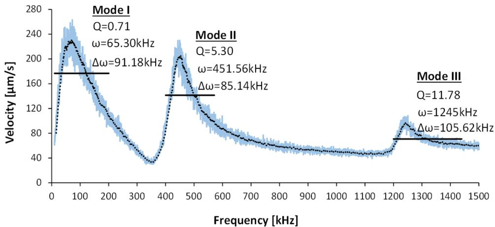
**Fig. 7.** Frequency response and the Q- factor for different bending modes of the cantilever with position- 0 of the acting electrode tested in ambient conditions.
