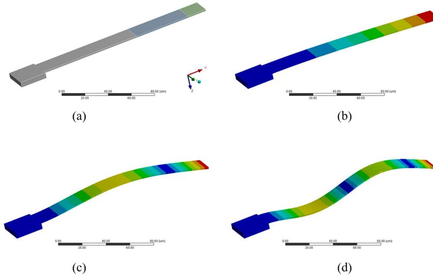
**Fig. 8.** The modal analysis of a polysilicon microcantilever. (a) geometrical model emphasizing electrode position; (b) the 1<sup>st</sup> mode; (c) the 2<sup>nd</sup> mode; (d) the 3<sup>rd</sup> mode of vibration with the acting electrode in position 1 (color online).
