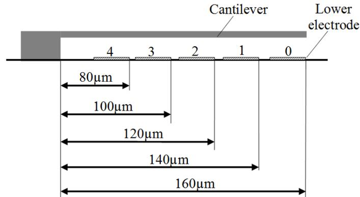
Fig. 3. Successive positions of the lower electrode.
