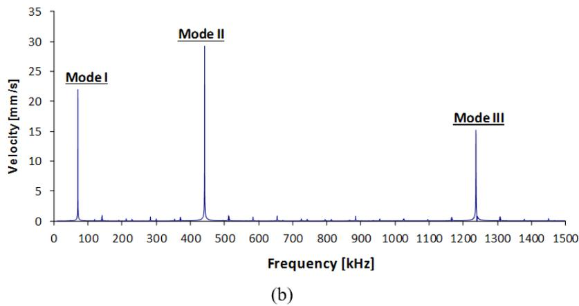
Fig. 10. Velocity of oscillations for different bending modes of the cantilever with the acting electrode close to the anchor in air (a) and vacuum (b).
