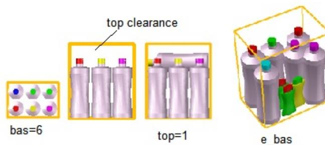
**Fig. 6.** Some possible layout configurations of the products
