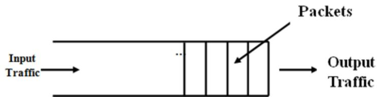
Fig. 12. Unlimited size buffer in the node.
