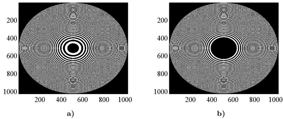
Fig. 2. Diffractive microlenses calculated for a focal distance 152 mm: a) integral; b) 3 central zones missing.
