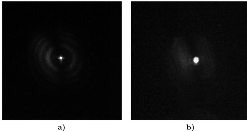
**Fig. 10.** Experimentally diffracted intensity obtained from the DML from Fig. 6 (entire) recorded at **a)**  $z = 40$  mm and **b)**  $z = 152$  mm.
