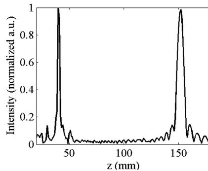
**Fig. 9.** Values on the optical axis from the simulated diffraction pattern given by the DML from Fig. 6.
