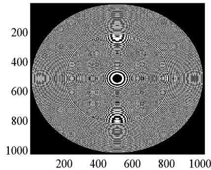
**Fig. 5.** The DML obtained after the combination of one FZP with the focal length 40 mm and one FZP with the focal length 152 mm and 16 missing central zones.
