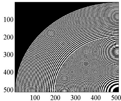
**Fig. 6.** A quarter from the DML obtained after the combination of: (1) one FZP with focal length 40 mm and (2) one FZP with focal length 152 mm and 17 missing central zones.
