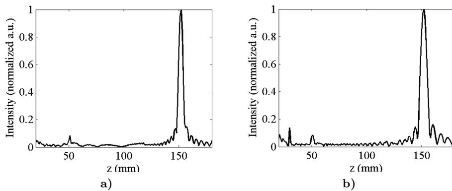
Fig. 3. Intensity along propagation axis calculated for FZPs with focal distance 152 mm: a) integral; b) 17 central zones missing.
