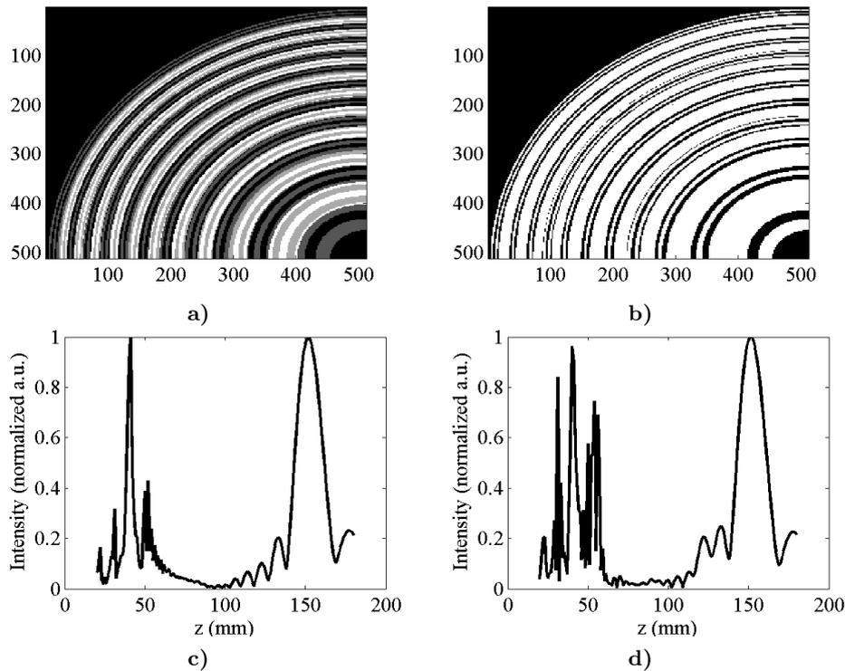
**Fig. 4.** The superposed DMLs obtained starting with the simple ones designed like in Fig. 1a and 2a with **a)** 4 levels; **b)** 2 levels; **c)** and **d)** the diffracted intensity along propagation axis with unwanted peaks from the DMLs designed like in Fig. 4a and b respectively.
