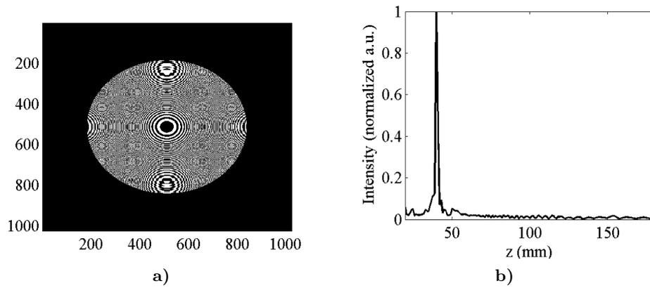
Fig. 1. a) FZP generated for a focal distance of 40 mm; b) intensity values on the propagation axis.
