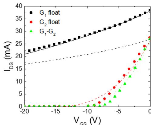
**Fig. 5.** Comparison of the experimental transconductances  $I_{DS} = f(V_{GS})$  of a dual-gates MESFET for  $V_{DS}=20$  V (symbol) in the 3 cases:  $G_1$  is floating,  $G_2$  is floating, and  $V_{G1} = V_{G2}$ . Dash line corresponds to numerical simulations. The solid line is calculated using  $V_{GS1} = 0.05 \times V_{GS2} + 1.8$ .
