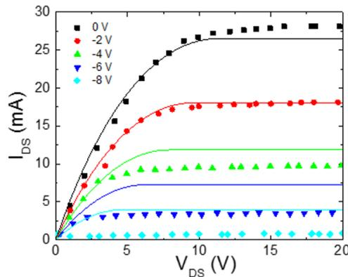
**Fig. 4.** Comparison of  $I_{DS} = f(V_{DS})$  curves between the analytical model (dots) and the measurement (lines) of the MESFET with  $V_{GS2} = 0$  V in theoretical curves and  $V_{G2}$  is floating in experimental ones.
