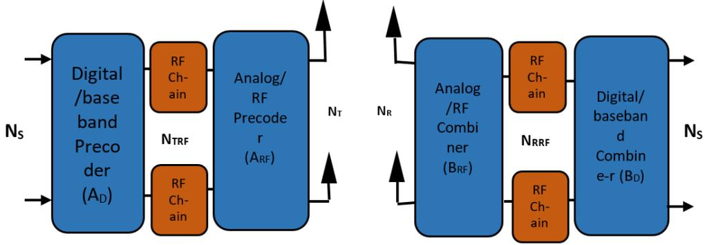
**Fig. 1.** Model of Millimeter-wave MIMO system.
