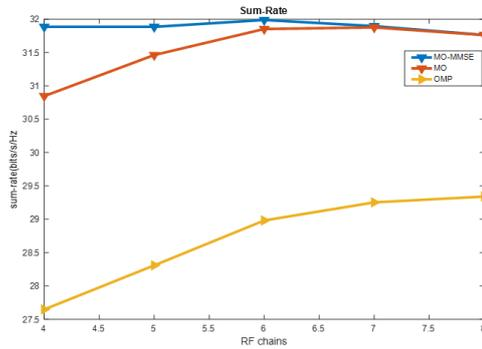
**Fig. 6.** Sum rate Vs. RF chains for 128\*64 System.
