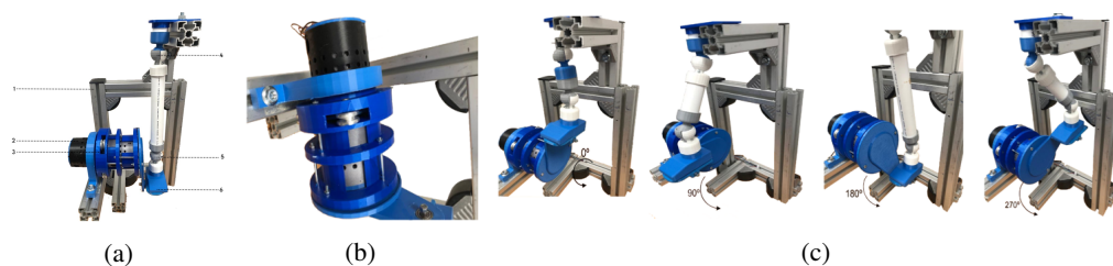
Fig. 4. (a): Experimental model for knee and ankle joint training: 1 – Aluminum profile metal frame; 2 – Stepper motor housing; 3 – Guide rollers; 4 – Knee joint; 5 – Ankle joint; 6 – Footplate support. (b): The actuation mechanism (c): Successive stages of knee and ankle joint movement simulation.
